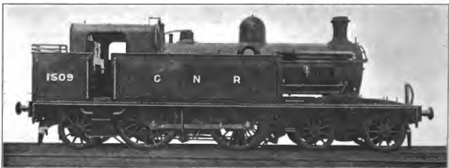
Fig. 5058. Ten-Wheel, Four-Coupled Tank Locomotive. Great Northern Railway. Cylinders 18 in. x 26 in.; Working Steam Pressure 170 lbs. per sq. in.; Total Heating Surface 1,123.8 sq. ft.; Diameter of Drivers 68 in.; Weight on Drivers 80,308 lbs.; Total Weight 138,770 lbs.
